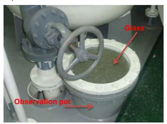
The drainage pot observation glass failed when the drainage pot was subjected to significant air pressure (about 30 bar) from the pressurised air receiver. Pressure accumulated in the drainage pot when liquid from the air receiver restricted the flow of air and liquid out of the pot into the drainage piping and bilge.
