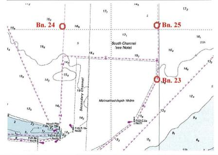
Pile driving for each beacon will take approximately one day with permanent features, including top marks, day marks and lights, to be installed the following day. Beacon piles will be marked overnight with temporary flashing lights, as detailed below:
